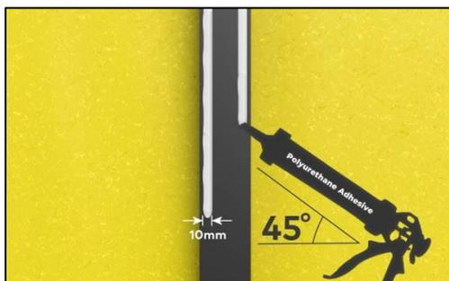
3. Applying polyurethane adhesive on the vertical profile
