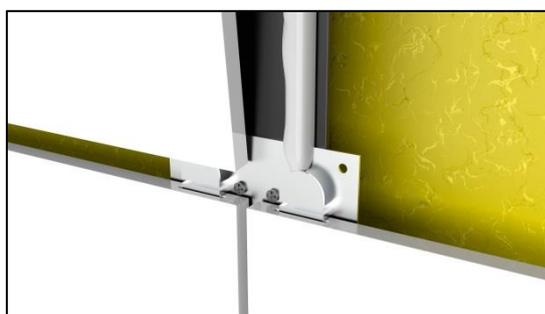
6. Inserting top clip and fixing the ceramic tile
